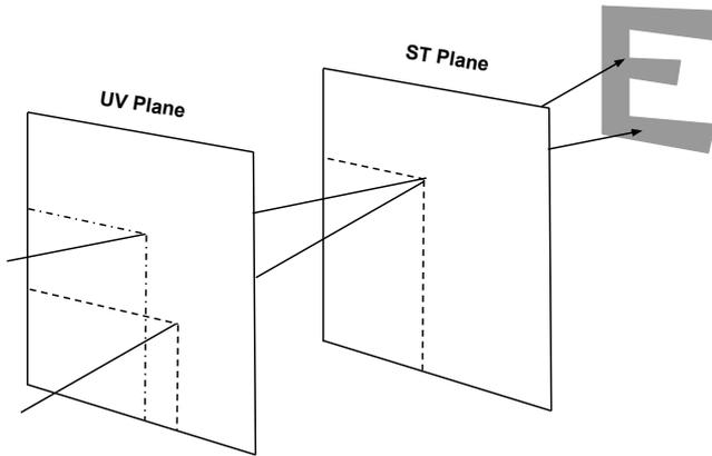
**Figure 1:** The light slab is a two-plane parameterization of the set of rays in a light field. The st-plane can be thought of as a collection of perspective images of the scene, while the uv-plane corresponds to the position of the observer.
