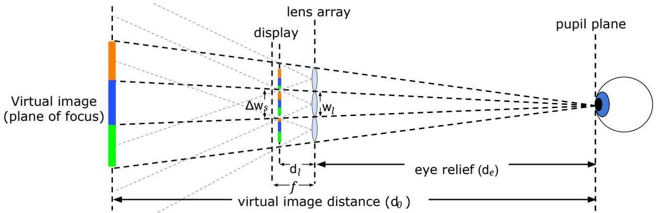
**Figure 2:** The Near-Eye Light Field Display; a microlens array is placed in front of the display and the human eye optically reconstructs the virtual image from the rendered 2D light field image
