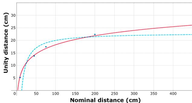
**Figure 4:** Graph showing the two proposed curves (red: see Equation 8, cyan: see Equation 9) for converting real distances to the equivalent virtual distances. Also shown are the points the curves are fitted to, one additional measurement was made at optical infinity that is not shown on the graph (the Unity distance had not changed from the previous measurement at 200cm).
